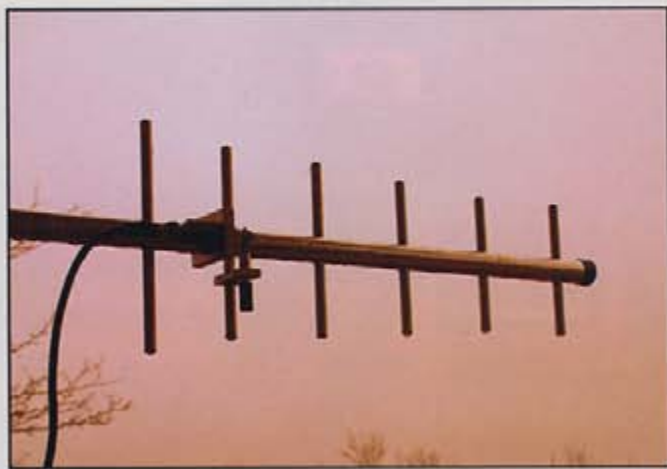
Here's my compact beam antenna useful for frequencies above 800 MHz. This is a surplus antenna originally designed for 800-MHz trunking radio repeaters. "Compact" is the key word in selecting antennas to be mounted in a relatively small area like an apartment balcony.
