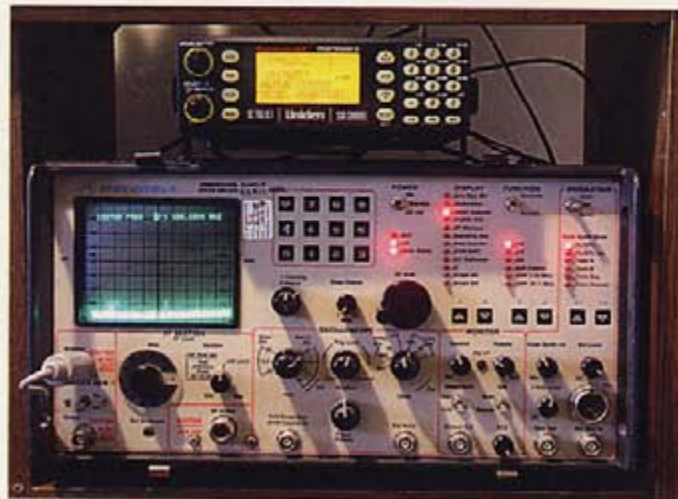
KITCHCOM's BC-780 sits upon the Motorola R2001D Communications System Analyzer. Together they are a potent pair of communication interception tools.
