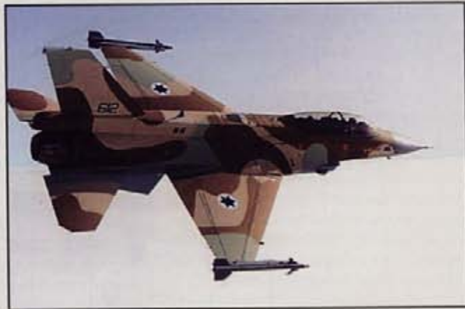
The F-16I looks radically different from other F-16s, with conformal fuel tanks, dorsal spine, and numerous fairings and bulges for undisclosed equipment.
